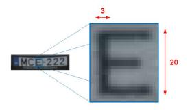
For optimal ANPR/LPR results, the most important factor is the size of the characters on the image. For Latin characters it is recommended to have an average character height of at least 16 pixels. For Arabic or other special characters, it is recommended to have characters that are at least 20 pixels in height. A higher resolution is needed in the latter case as these characters are more intricate in their design.
